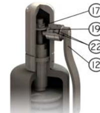
Palanca estanca Sealed packing lever
